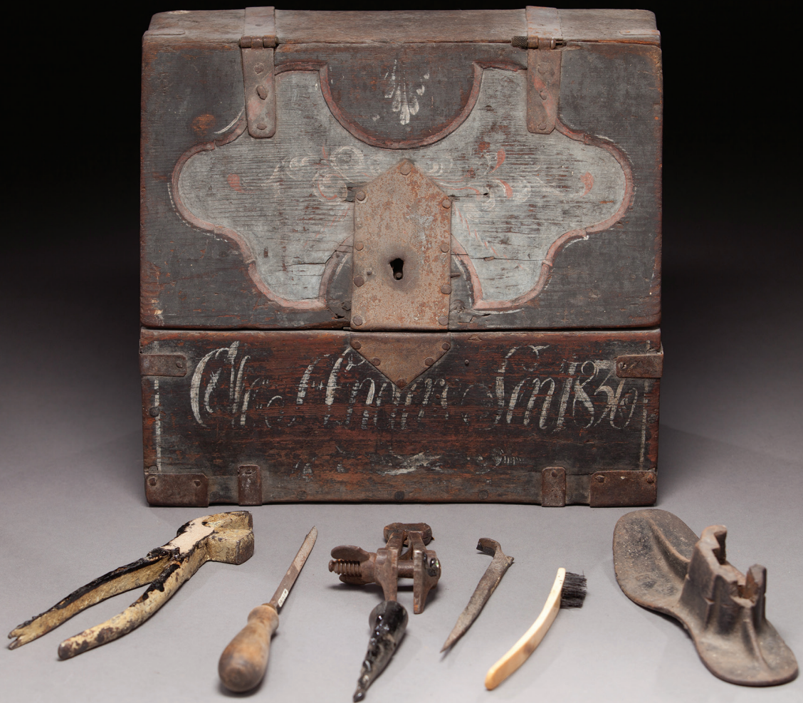
Ole A. Lomen's toolbox was embellished with rosemaling in 1836. He and wife Marit Knutson came from Vestre Slidre, Valdres, to Koshkonong, Wisconsin, in 1848 and moved on to Winneshiek County, Iowa, in 1850. Tools stored in the box would have been used in making and repairing leather shoes and include lasting pinchers (left) and lasting jack (right) along with other hand tools for shaping and finishing the leather. 16 Vesterheim 1979.017.001 – Gift of Oscar Lomen.
