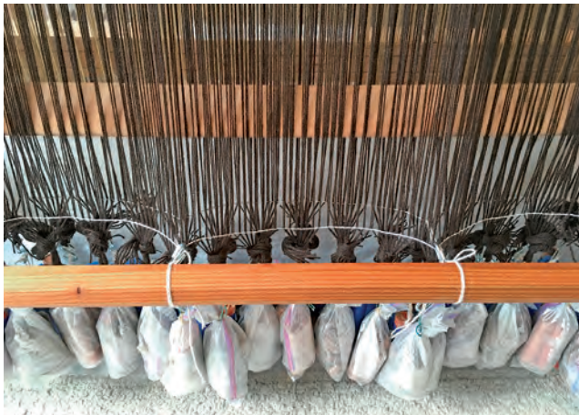
Fig. 5: Weight-rows in the coverlet-width warp, configuration 4: the two forward-layer rows are attached by their spacing chains to the shed rod; a pattern board is stored in the warp threads above (Image: Katherine Larson)
