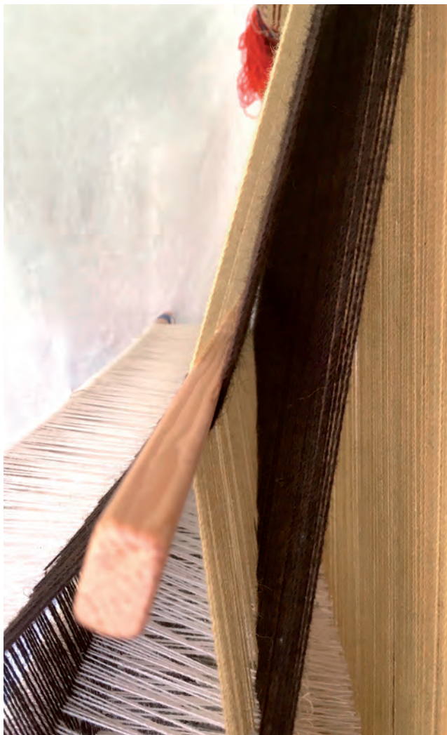
Fig. 2: Pattern sheds are formed at the front of the loom when weaving double-cloth: a forward-layer pattern shed is open immediately behind the pattern stick; back-layer pattern warps (gold) are held on the pattern stick in front of the open shed (brown warps); back-layer background warps (gold) remain behind (Image: Katherine Larson)
